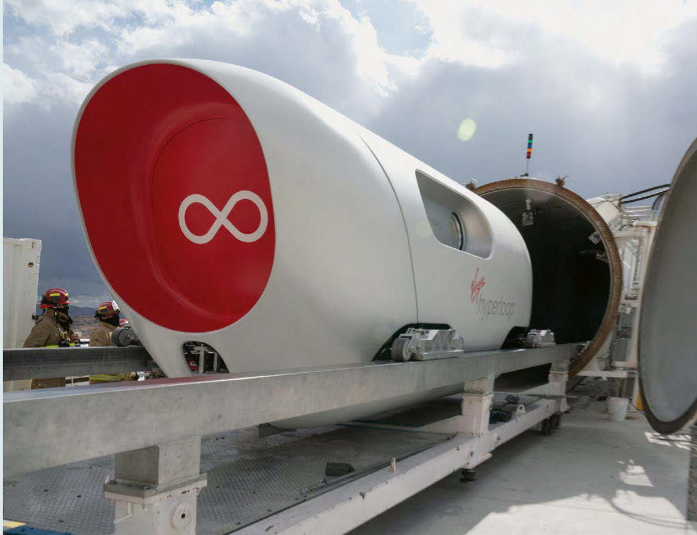
On a 500-meter-long test track in Las Vegas, Nevada, the two-seater Pegasus has already reached a top speed of 172 kilometers per hour with passengers.
