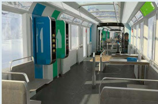
The cars can be equipped with different service modules such as vending machines for beverages, snacks, or tickets.
