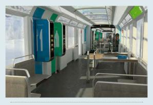
The cars can be equipped with different service modules such as vending machines for beverages, snacks, or tickets.
