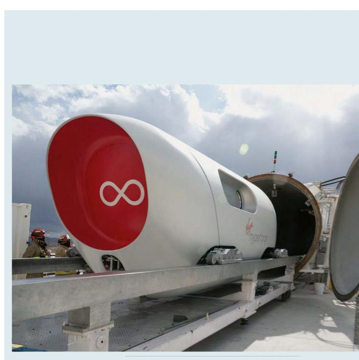
On a 500-meter-long test track in Las Vegas, Nevada, the two-seater Pegasus has already reached a top speed of 172 kilometers per hour with passengers.
