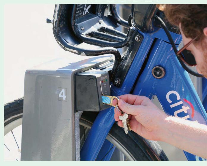
The personal RFID keys are used to unlock the bikes at the stations.
