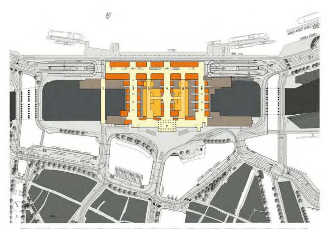
Floor plan of Amsterdam Central Station: 1 Cuypers Passage (low-speed transit corridor), 2 West Tunnel, 3 IJ Passage, 4 Middel Tunnel, 5 Amstel Passage, 6 East Tunnel, 7 Cuypers Hall
